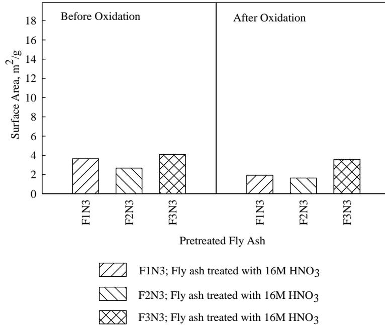
**Figure 3.8:** Type of Fly Ash Effect on Oxidation
