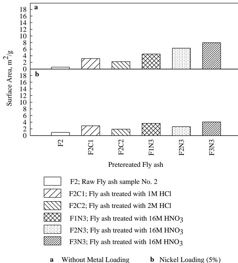
**Figure 3.5:** Effect of Metal Loading on Surface Area of the Catalyst
