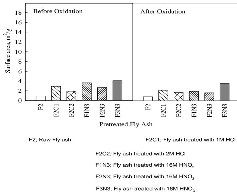
**Figure 3.9:** Variation in Surface Area of the Catalysts during Different Experimental Conditions
