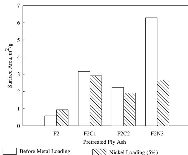
**Figure 3.4:** Effect of Different Acids Pretreatment and Metal Loading on Surface Area of the Synthesized Catalysts
