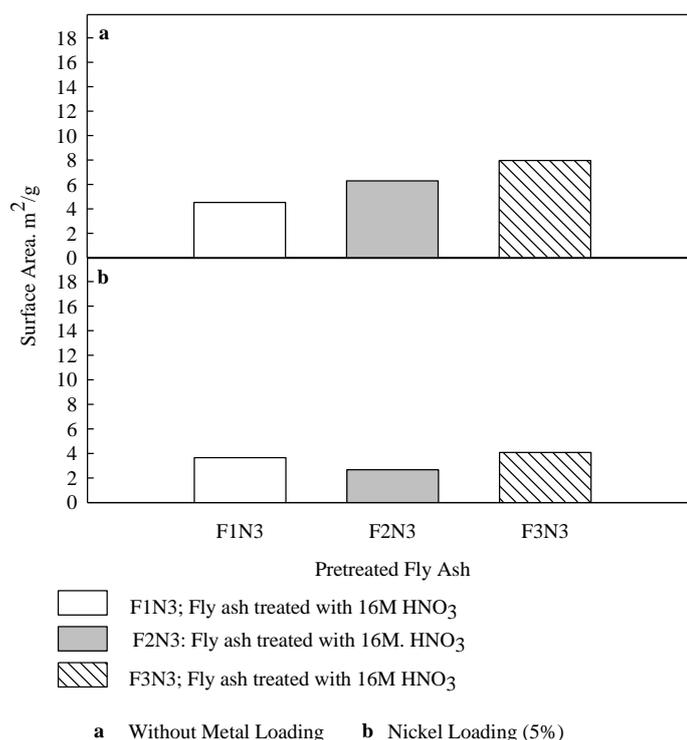
**Figure 3.3:** Effect of Type of Fly ash on Surface Area after Pretreatment with Nitric Acid and Metal Loading
