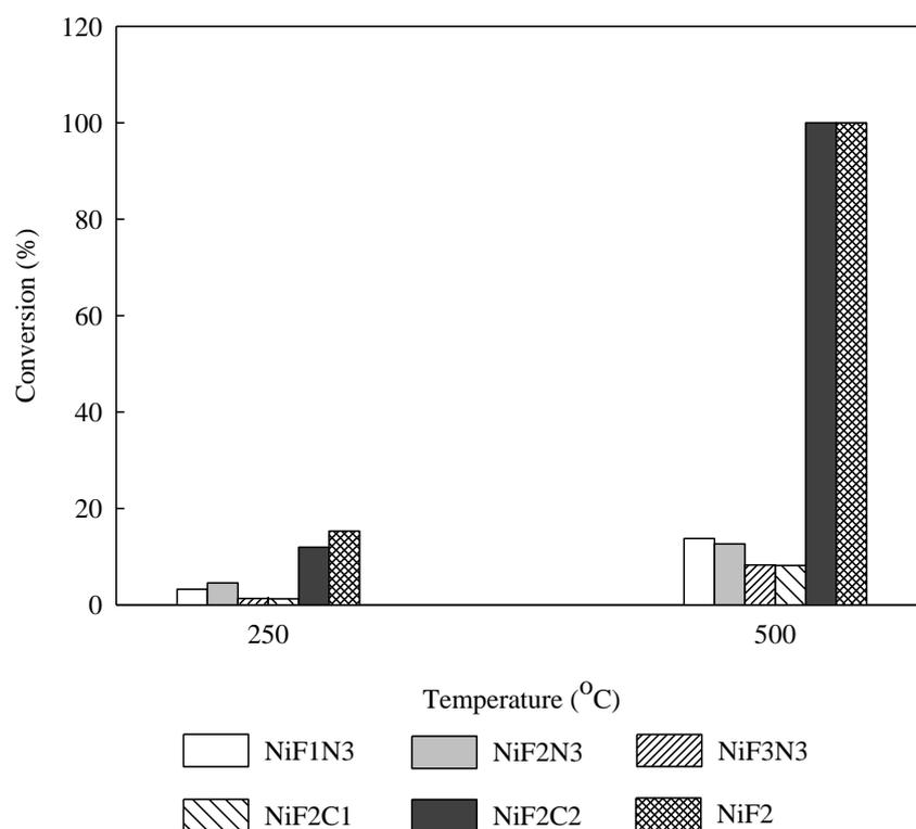
Figure 3.6: Oxidation of CO using Nickel Catalysts
