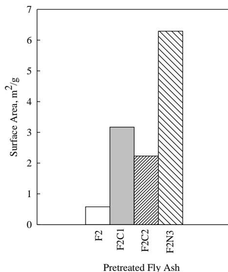
**Figure 3.2:** Enhancement in Surface Area of Fly ash on Acid Pre-treatment
